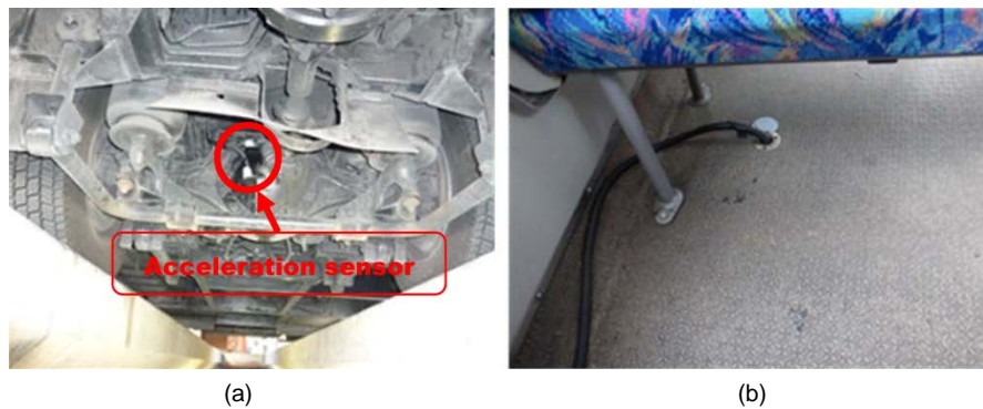
Figure 14. Installation of acceleration sensor to the bus (vehicle). (a) Acceleration sensor installed to the rear wheel of the bus; (b) Wiring routes into the bus.
