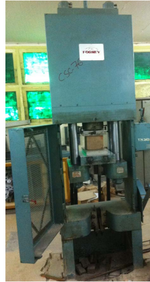
Figure 3. Compressive strength test is being performed on a baked clay cube of 150 mm size, using universal testing machine.
