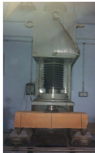
Figure 4. A plain baked clay beam is being tested for modulus of rupture in universal beam testing machine.
