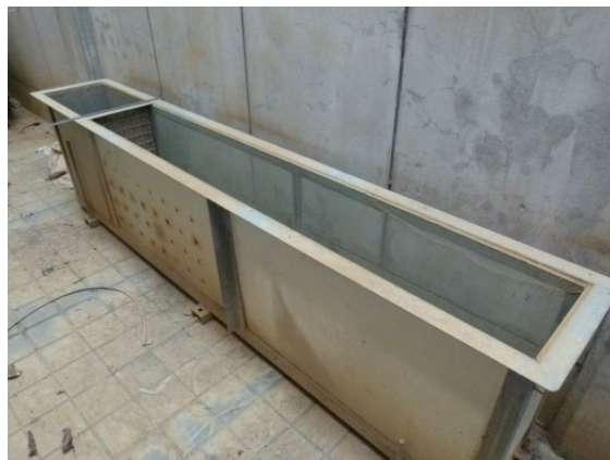
Figure 3. Photo of hydraulic model experiment channel.
