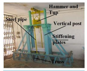
Figure 4. Drop weight impact testing machine.
