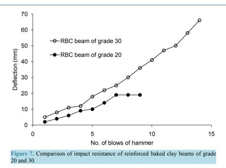
impact resistance as compared to the grade 20 beams. This is because, 1) the beam of grade 30 failed due to yielding of a steel bar followed by crushing of baked clay, and 2) the beams of grade 20 failed due to crushing of baked clay material. This behaviour of the RBC beams is consistent with that of RCC beams, see e.g. Khan [22].
