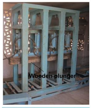
Figure 2. Wooden plunger used to compress clay beams in mechanized system.
