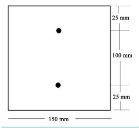
Figure 3. Cross section of reinforced baked clay beam.
