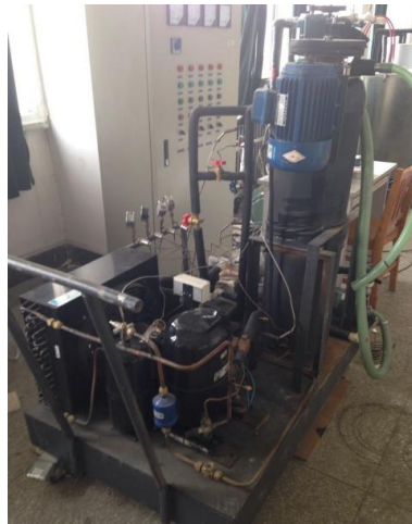
Figure 2. Prototype of the dynamic ice slurry preparation unit.
