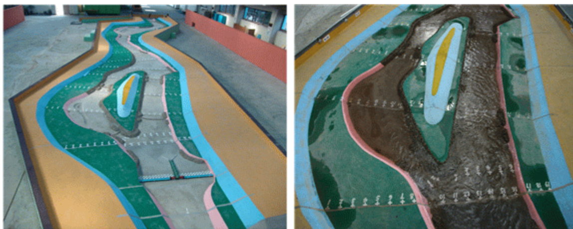
Figure 3. Channel reproduction for hydraulic model experiment.
