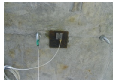
Figure 2. Acceleration measurement in Seongdong viaduct. (a) Layout of accelerometers; (b) View of installed accelerometers.
