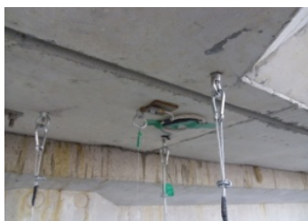
Figure 1. Acceleration measurement in Gomo viaduct. (a) Layout of accelerometers; (b) View of installed accelerometers.
