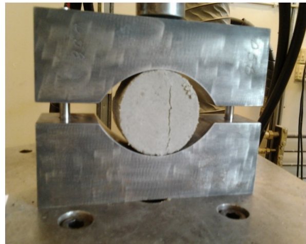
Figure 5. Test arrangement with typical tensile fracturing of brittle material (Portland concrete).
