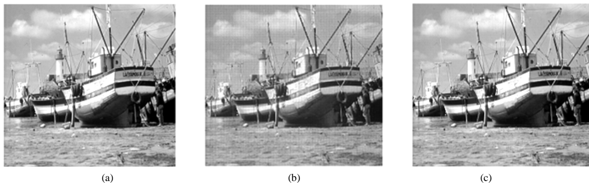
Figure 4. (a) Original "Boat" Image; (b) Reconstructed image with ( 8 \times 16 ) NPR CMFB filter bank; (c) Reconstructed image with ( 8 \times 24 ) NPR CMFB filter bank.
