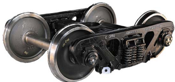
Figure 3. Bogie suspension system [19].
