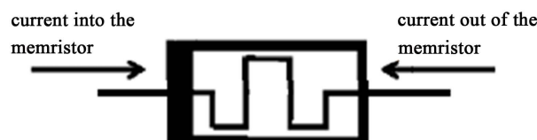
Figure 1. Memristor symbol. Thick black line on the left represents the polarity of the device. If current flows into the device, resistance of the memristor decreases and vice versa.
