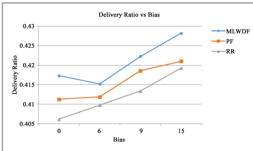
Figure 8. Packet delivery ratio performance comparison for various bias values using MLWDF, PF and RR schedulers.
