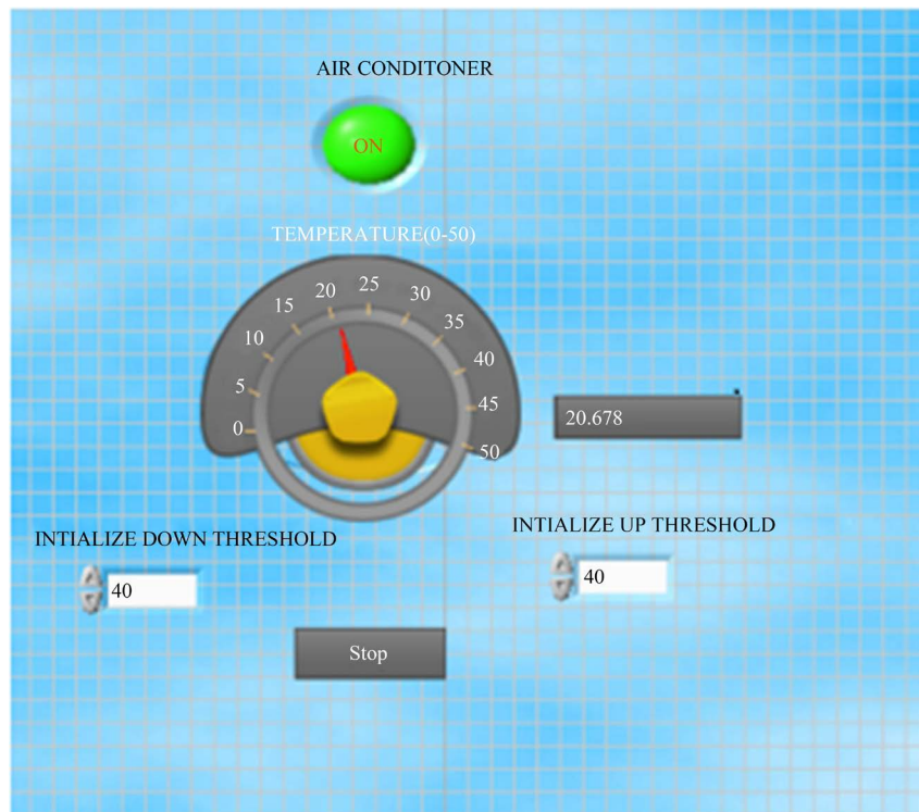
Figure 5. Air conditioner controller based on threshold values (input by consumer).
