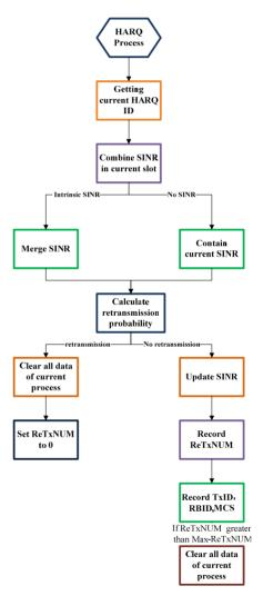
Figure 2. Flow chart of synchronous HARQ for D2D.
