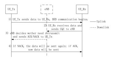
Figure 1. Flow chart of synchronous HARQ for D2D.
