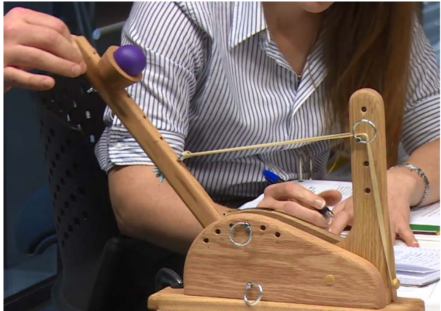
Figure 2. Illustration of the Statapult® Catapult system shown in use by one of the authors.
