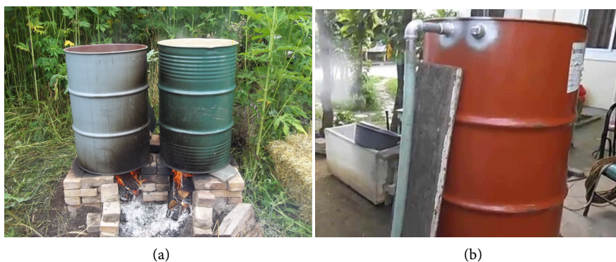
Figure 6. Conventional autoclave process by using barrels; (a) Steam generation and media storing in same barrel; (b) Separate barrels used for steam generation.
