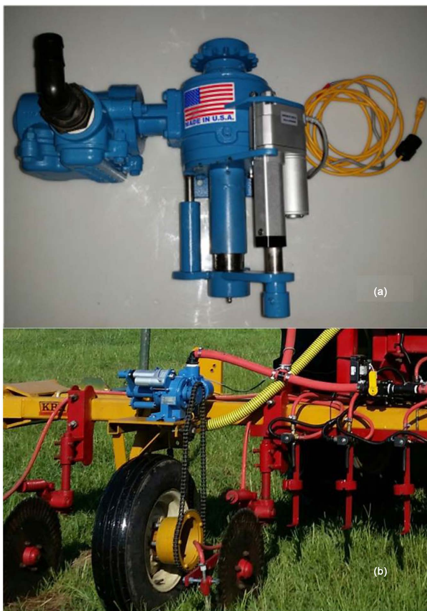
Figure 2. (a)The Clemson electro-mechanical controller, retrofitted to a John Blue piston pump (b), KBH nutrient applicator.
