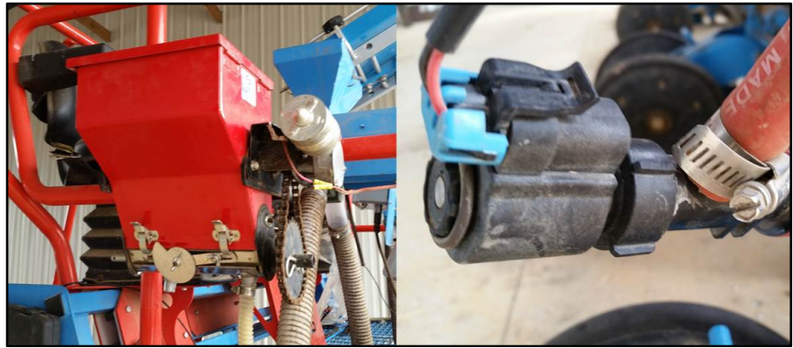
Figure 5. The Gandy granular hoppers (left), and the TeeJet 55280 e-Chemsaver, electric solenoid shutoff valves (right).
