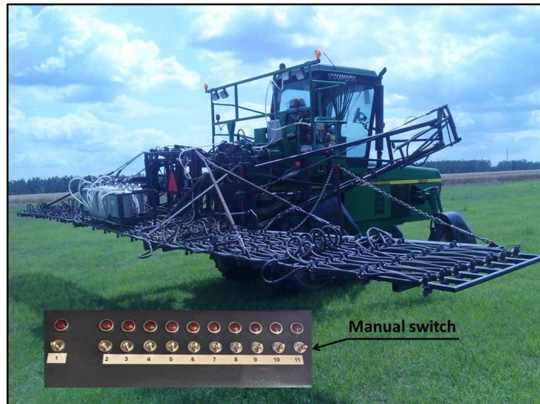
Figure 1. A multi-boom sprayer and the manual switches for controlling booms 1 to 11.
