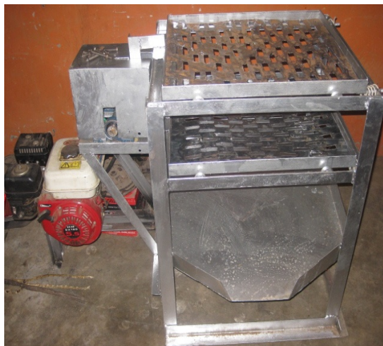
Figure 1. Groundnut in-shell grader.
