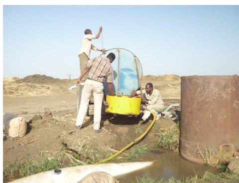
Figure 3. Injection of the dissolved urea fertilizers into the irrigation water by means of pressure differential tank system.
