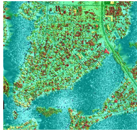
Figure 7. Identified clusters in the LiDAR dataset using the sweeping spatial clustering algorithm (Intended for color reproduction).
