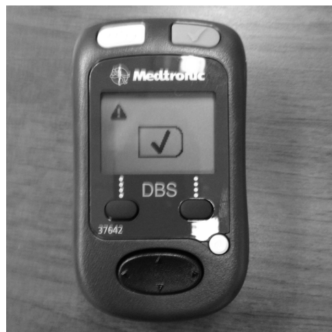
Figure 2. Deep brain stimulation patient programmer for setting status to "On" and "Off" mode.
