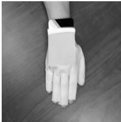
Figure 1. Smartphone mounted to the dorsum of the hand by a latex glove.
