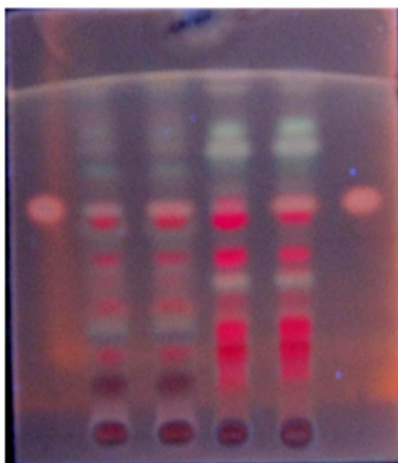
Figure 2. TLC plate showing fluorescent bands visualized in the Camag Scanner 4. Lanes: 1 and 6—Standard, 2— A. pallens leaves, 3— A. pallens leaves spike, 4— A. nilagirica (Kolhapur) leaves, 5— A. nilagirica (Kolhapur) leaves spike.
