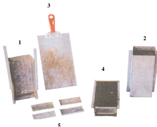
Figure 1. Columns techniques used for leaching experiments: 1, empty half column; 2, complete column full of soil; 3, special spatula to divide the column; 4, a half column ready for sowing test plants; 5, stoppers [1].
