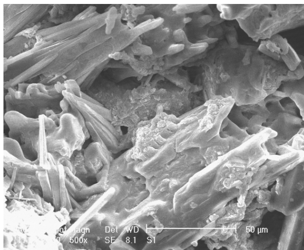
Figure 4. Solid bridges and mechanical interlocking bonds between compost and urea particles.
