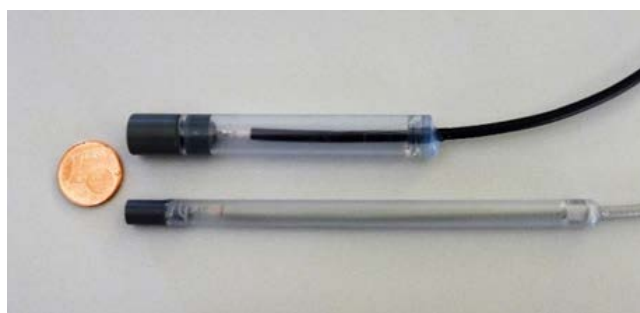
Figure 2. Graphite paste ion-selective electrodes of different dimensions.
