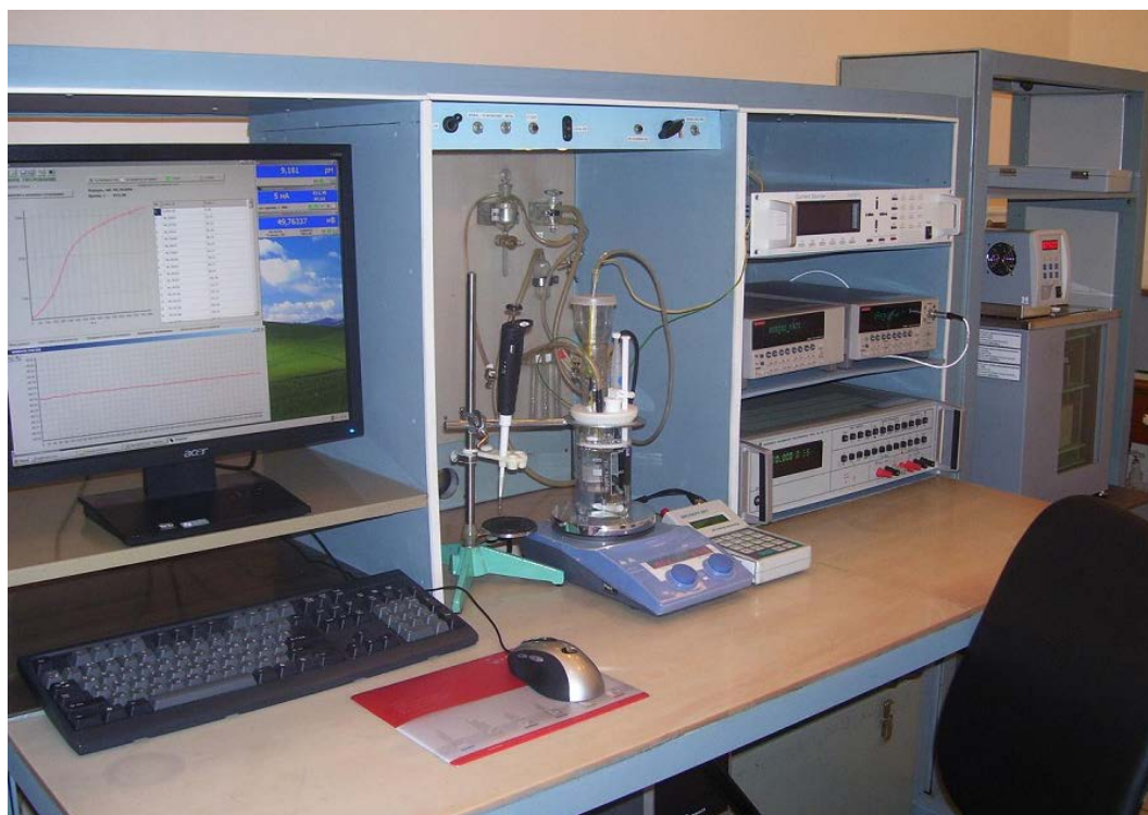
Figure 1. An external view of the “State primary standard of the units of mass (molar) fraction and mass (molar) concentration of the component in liquid and solid substances and materials based on coulometric titration method GET 176-2010”.
