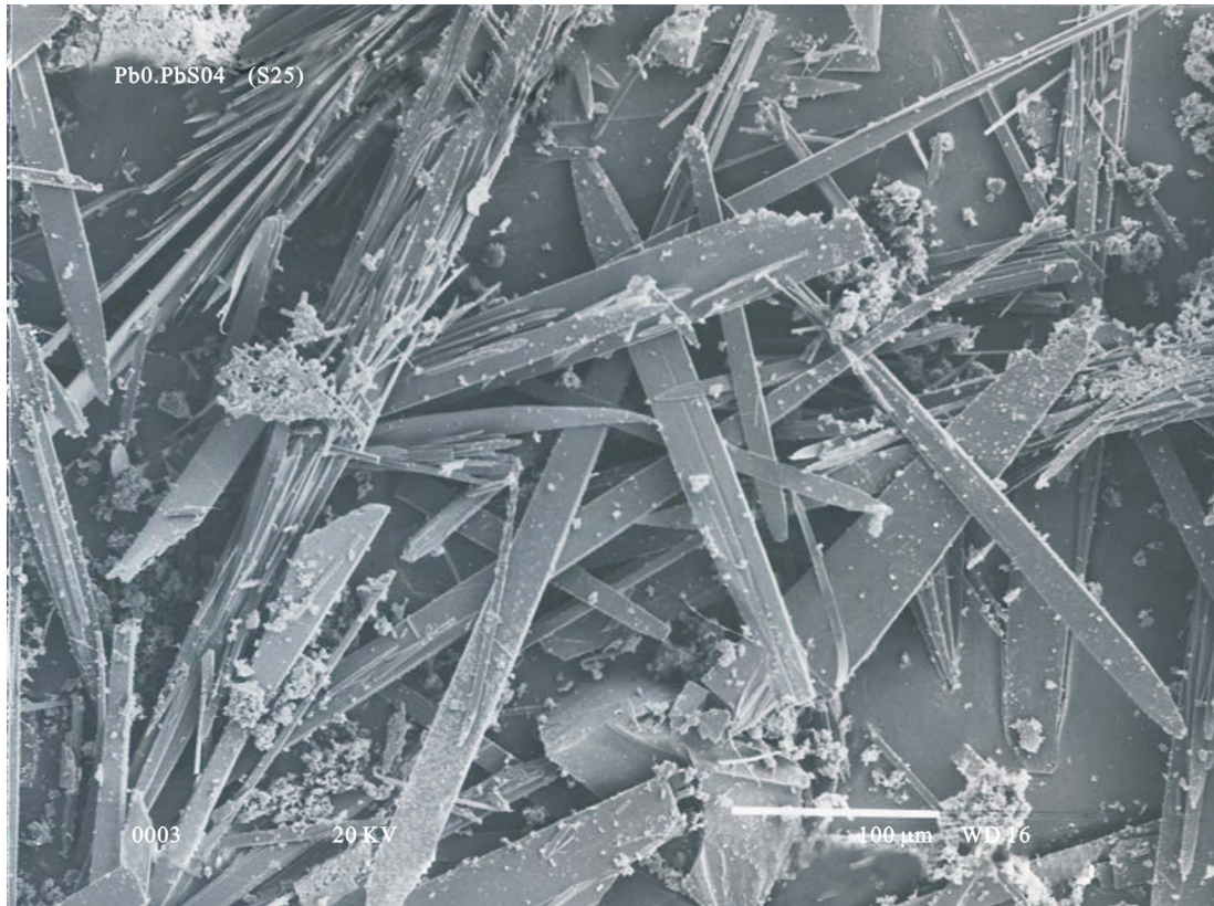
Figure 4. SEM electron microscopic photograph of \text{PbSO}_4/\text{PbO} , enlargement is 200 \times .
