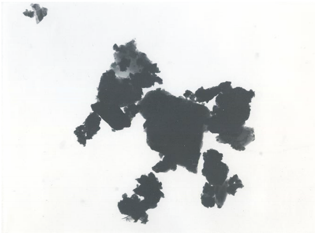
Figure 5. TEM electron microscopic photograph of \text{PbSO}_4/\text{PbO} , enlargement is 20000 \times .
