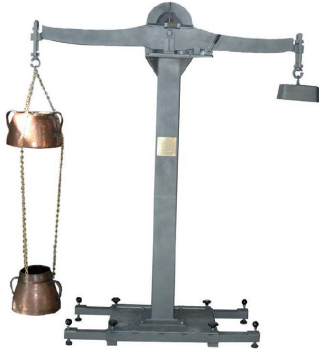
Figure 1. A physical reproduction of Galileo's two-bucket setup. This model is found at the University of Pavia, Italy (Caffarelli, 2009: p. 9).
