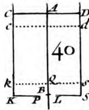
Figure 9. Vessel with an aperture made in the bottom, for which Equation (15) was developed (a reproduction of Figure 40 from the Traité de l' équilibre et du mouvement des fluides ).
