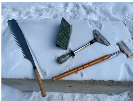
Figure 35. Hand Tools. They haven’t changed much over the millennia: saw, chisel, scraper, tined fork ... except that today we can enjoy the magnificence of Japanese tool steel for the blades. Photo by R.S.N., January 2019.
