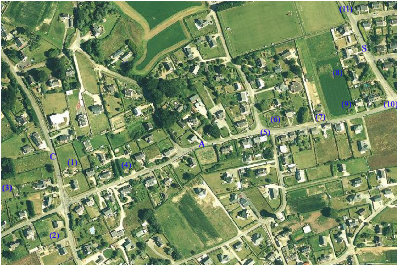
Figure 1. Saint-Pabu radar camp components: (1) 1 st V2a and L410A , (2) 1 st Freya radar emplacement, (3) 1 st Würzburg-Riese radar emplacement, (4) L479 Anton , (5) bunker Vf integrated in a modern house, (6) area hosting camp components, (7) 2 nd Freya radar emplacement, (8) Vf bunker covered with terrain and tobruck, (9) 2 nd V2a , (10) East camp entrance, (12) 2 nd Würzburg-Riese radar emplacement, A rue Avel Vor, C rue Corn ar Gazel, S rue du stade [Geoportail].
