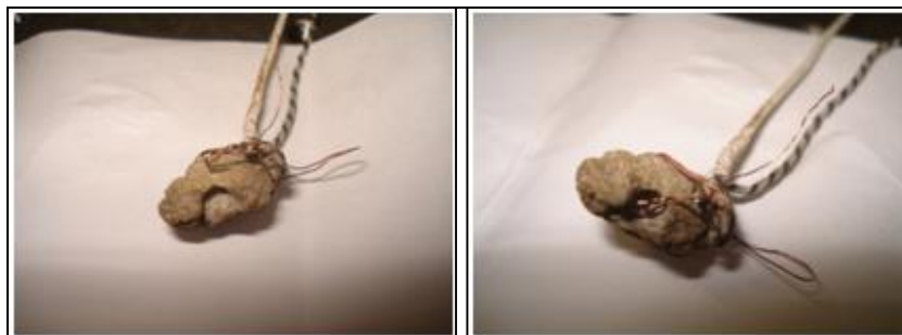
Figure 2. J-type thermocouple installed in the cavity of material recovery for TL.
