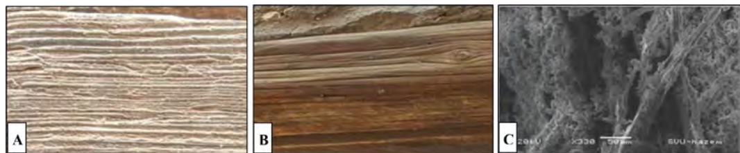
Figure 7. ((A), (B)) The window lintels in the outer portico showing the roughness of weathered wood surface, (C) the accumulated dust particles between the wood fibers, SEM micrograph. 50 \mu m.
