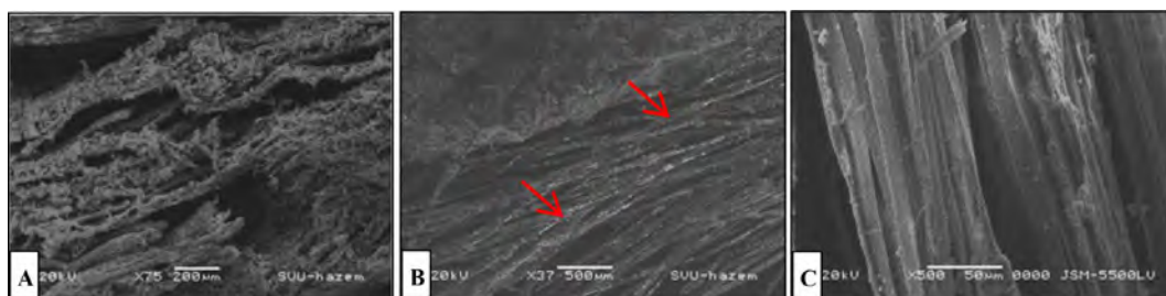
Figure 10. SEM micrographs of the door lintel in the mausoleum dome chamber, (A) a longitudinal section showing the fragile and detached wood fibers, (B,C) a longitudinal section showing the detached wood tracheids. (bar: (A) 200 μm, (b) 500 μm, (C) 50 μm).
