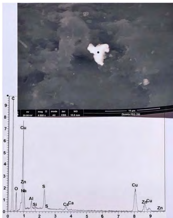
Figure S2. A plaque of brass, located on hair number 3. Above: SEM photograph (in CBS, 4000×) of the plaque. Below: spectrum at the black point. C: carbon; O: oxygen; Cu (three peaks): copper; Zn (three peaks): zinc; Na: sodium; Al: aluminium; Si: silicon; S (two peaks): sulphur; Ca (two peaks): calcium.
