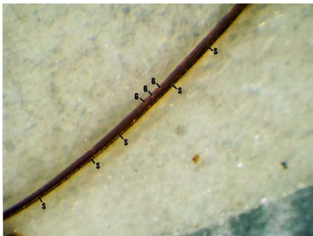
Figure 1. Optical view (20×) of a portion of hair number 2. S: silver; G: gold.
