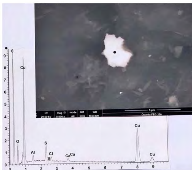
Figure S1. A plaque of copper, located on hair number 3. Above: SEM photograph (in CBS, 8000×) of the plaque. Below: spectrum at the black point. C: carbon, O: oxygen; Cu (three peaks): copper; Al: aluminium; S (two peaks): sulphur; Cl: chlorine; Ca (two peaks): calcium.
