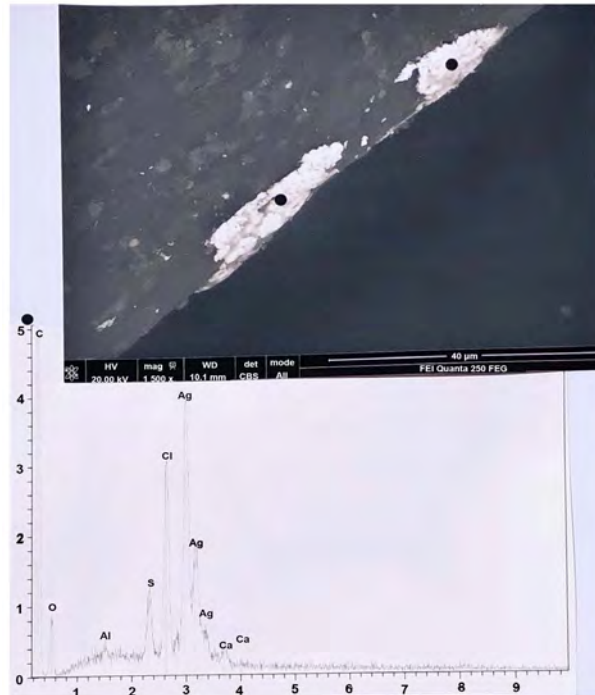
Figure 3. Two other deposits of silver chloride on hair number 2. Above: SEM photograph (in CBS, 1500×) of the two deposits. Below: spectrum at the black points.
