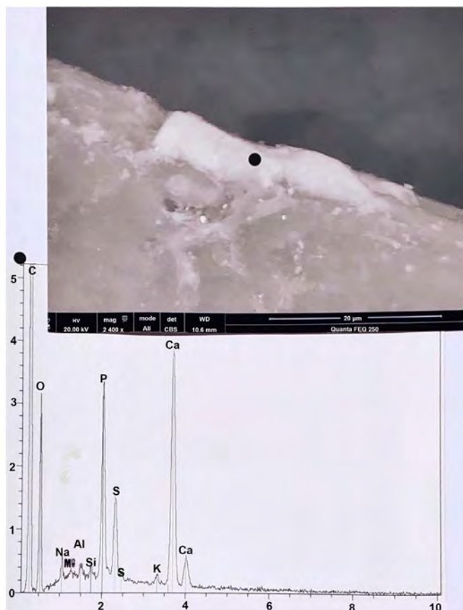
Figure 19. Example of a bone scale (in another part of hair 3). Above: SEM photograph (in CBS, 2400×) of the bone scale. Below: spectrum at the black point. C: carbon; O: oxygen; Na: sodium; Mg: magnesium; Al: aluminium; Si: silicium; P: phosphorous; S (two peaks): sulphur; K: potassium; Ca (two peaks): calcium.
