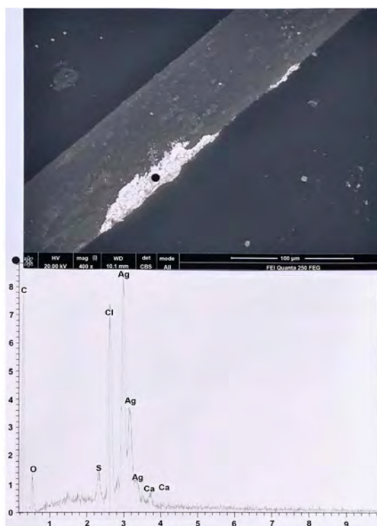
Figure 2. One deposit of silver chloride on hair number 2. Above: SEM photograph (in CBS, 400×) of the deposit (the black point indicates the location where EDX analysis is realized). Below: spectrum at the black point. C: carbon; O: oxygen; S: sulphur; Cl: chlorine; Ag (three peaks): silver; Ca (two peaks): calcium.
