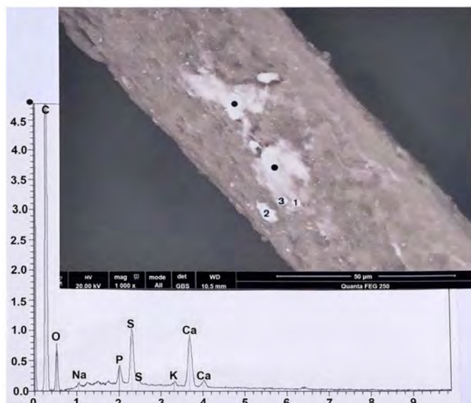
Figure 17. An example of a thin deposit of calcium phosphate, located in some part of hair number 3. Above: SEM photograph (in CBS, 1000 \times ) of the deposit (1-3: calcite particles). Below: spectrum at the black points. C: carbon; O: oxygen; Na: sodium; P: phosphorous; S (two peaks): sulphur; K: potassium; Ca (two peaks): calcium.
