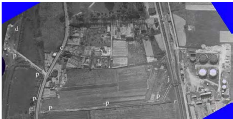
Figure 8. oil pipeline—c: rue Chevière; d: oil dock; s: pumping station on bollard c; p: pipeline; j: pipeline metal bridge on the SNCF railway; r: SNCF railway; t: oil terminal. (Mission identification: C1522_0281_1954_CDP860_0358, cliché n°358, scale: 1/4090, cliché type: Argentique, Date de prise de vue: 12/04/1954).
