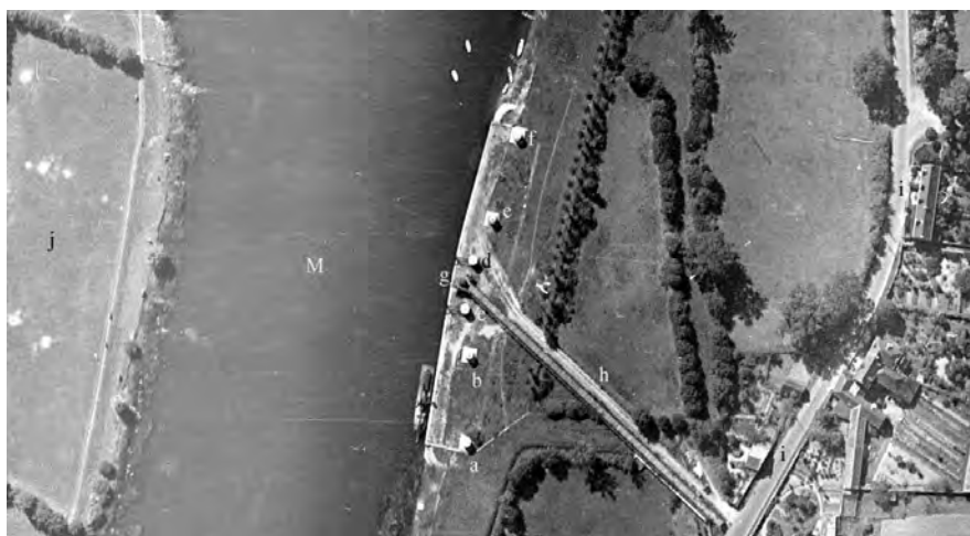
Figure 6. Bouchemaine oil dock—a, b: main columnar bollards; c: disappeared main columnar bollard; d, e, f: main columnar bollards; g: pumping station; h: dock's access road—pipeline road; i: actual rue Chevrière; j: possible bomb impact craters, M: Maine river. (Mission identification: C93PHQ8041_1948_CDP3032_0010, cliché n°10, scale: 1/5034, cliché type: Argentique, Date de prise de vue: 17/09/1948).
