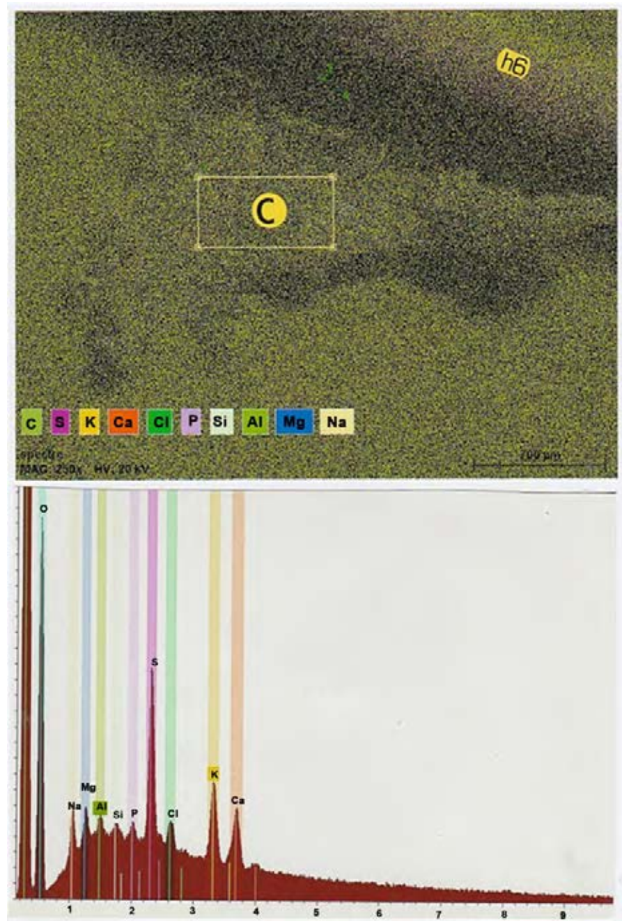
Figure 26. Map and general spectrum of structure C. Above: map of C (the general spectrum is taken in the rectangular area indicated); h6: the part of hair number 6. The coloured code of each element is indicated in the lower part of this map. Below: general spectrum of C (the upper limit of the lower red area indicates the background noise).
