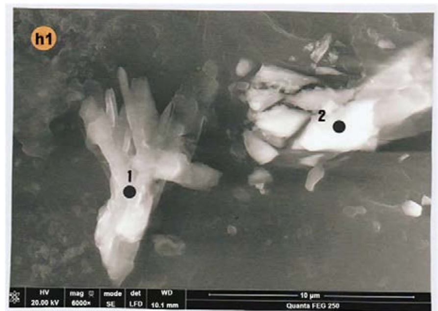
Supplementary Figure 4. SEM photograph (in LFD, 6000×) of micro-needles (1) and micro-plaques (2) of sulfate double of calcium and potassium, deposited on some part of hair number 1 (h1). Black spots indicate the locations where EDX analyses are realized.
