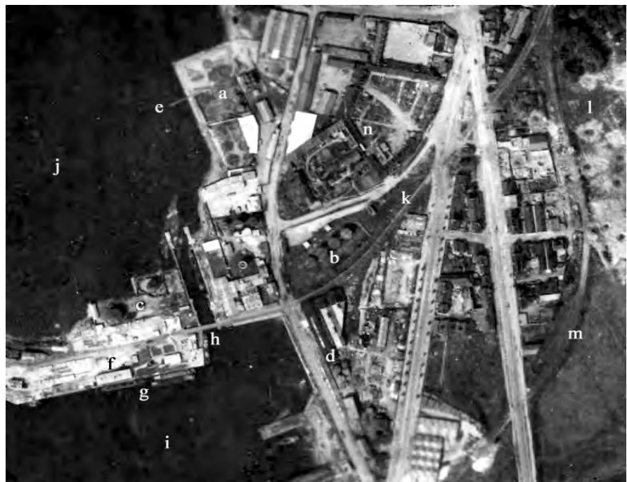
Figure 4. Talards oil terminal organization—a: 1st area—main tanks burned by the Howard-Johnson’s demolition group; b: 2nd area; c: 3rd area; d: 4th area, e: mooring pier; f: degaussing station (Tomezzoli & Pottier, 2016); g: moored barges; h: movable bridge; i: Bouvet basin; j: Jacques Cartier basin - Mare aux Canards; k: railway; l: bombed zone; m: railway; n: Talards casern. (Mission identification: C1115-0331_1944_106G1614_4005, cliché n 4005, scale: 1/10313, cliché type: Argentique, Date de prise de vue: 24/07/1944).
