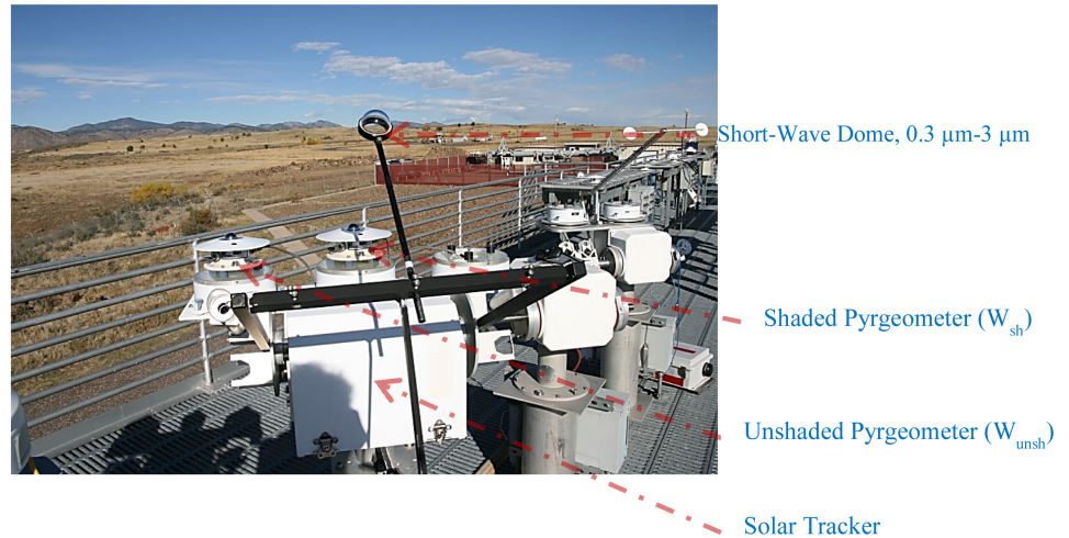
Figure 1. Set up of shaded and unshaded pyrheliometers to measure the longwave irradiance in solar beams.
