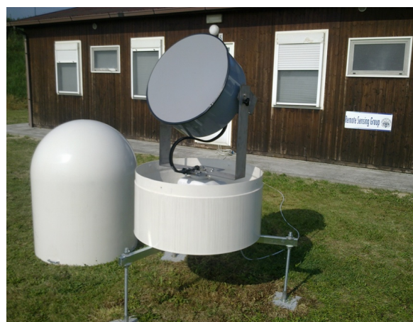
Figure 1. Short range X-band single polarization mini weather radar with high temporal and spatial resolution.
