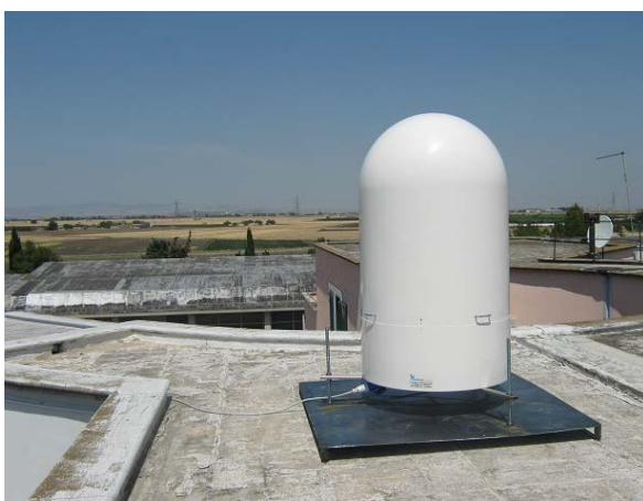
Figure 1. Short range X-band single polarization mini weather radar with high temporal and spatial resolution.
