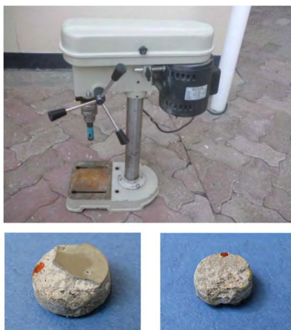
Figure 1. The coring instrument (top); and typical samples of proofed and unproofed cored discs (bottom left and right, respectively).
