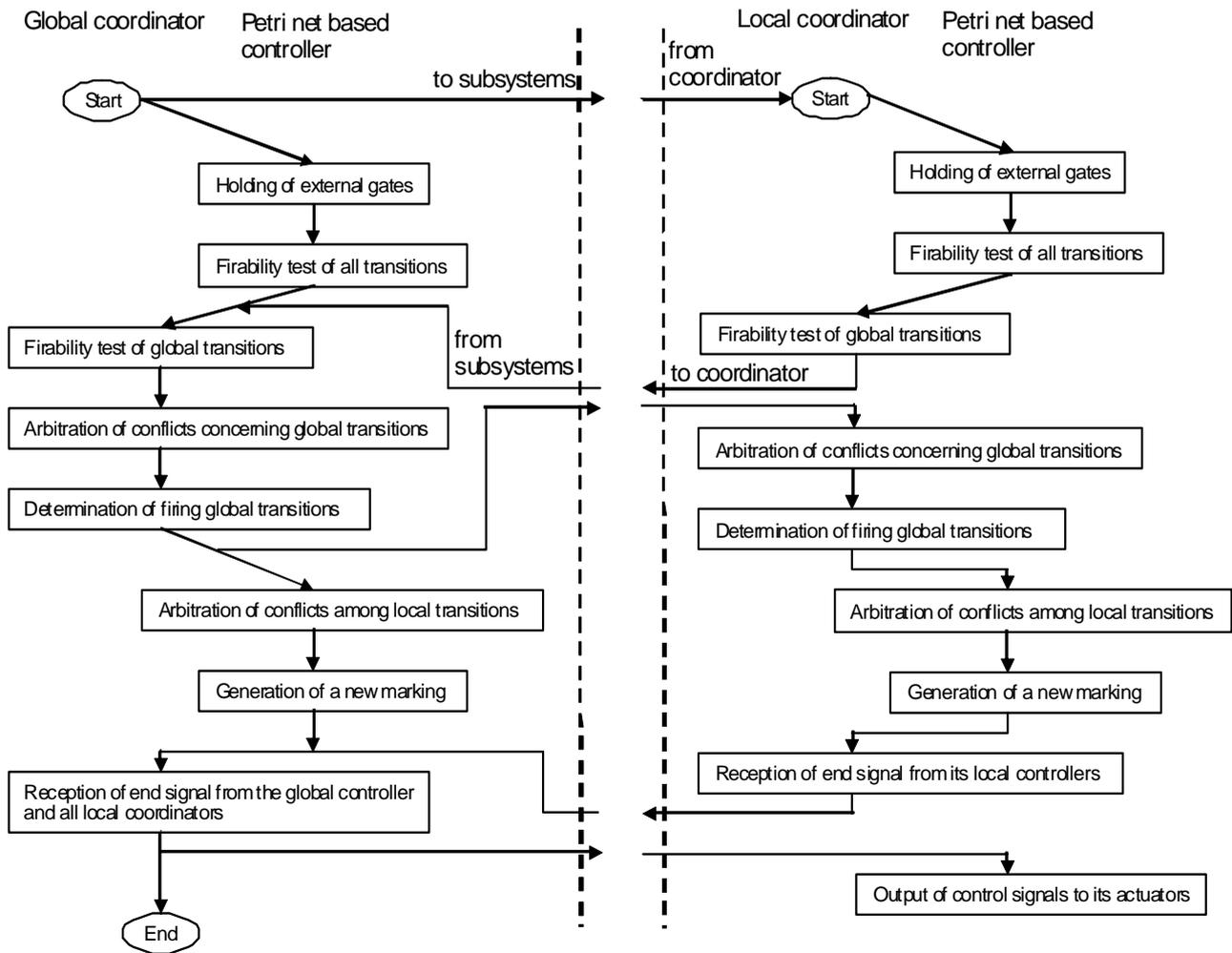
**Figure 7. Flowchart of coordination in two-level control system**
