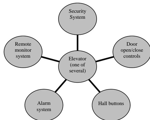
**Figure 1. An OV-1, high-level view of the interaction between several of the elevator's microprocessors and some of the other relevant computer-controlled systems**
