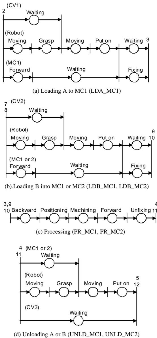
Figure 11. Detailed Petri net representation of subtasks
