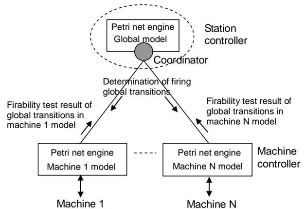
**Figure 5. Petri net based control structure with coordinator**
