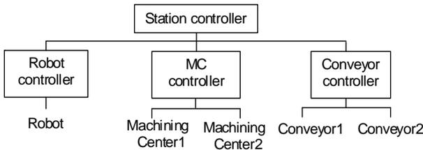
Figure 2. Example structure of distributed control system
