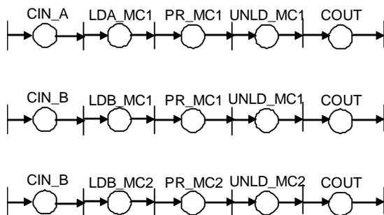
Figure 9. Petri net representation of the task specification of the example system
