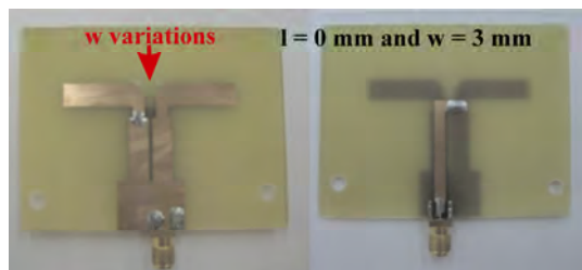
Figure 4. Printed dipole antenna for l = 0 mm and w = 3 mm. Top Layer (left) – Bottom Layer (right).
