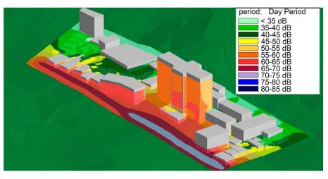
**Figure 4.** Three-dimensional noise mapping of the frontal façades of the buildings of the University Hospital of the Federal University of Paraná—UFPR.
