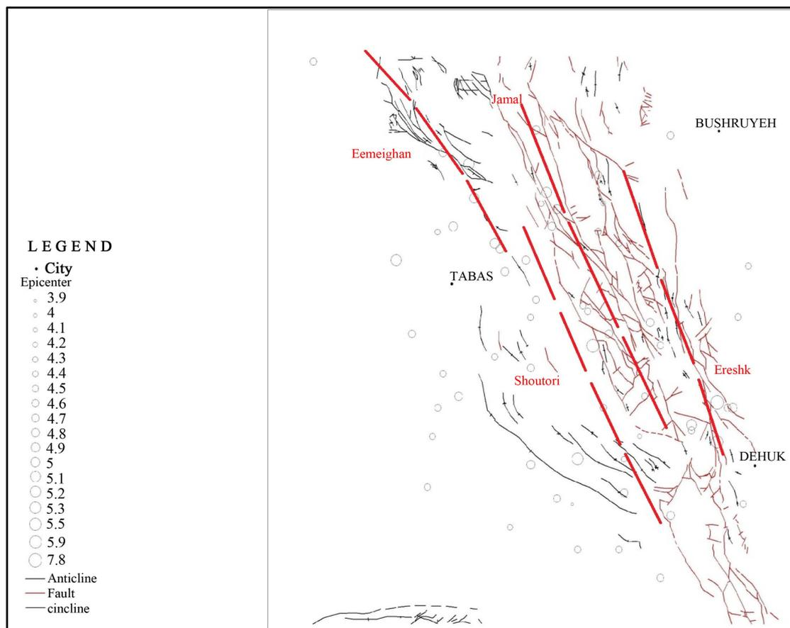
**Figure 8.** Seismic records and the major structural front traces of study area.
