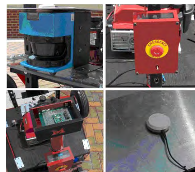
Fig. 14 Specialized mounts: laser ranging system (top left), safety switch (top right), digital compass (bottom left), and GPS antenna (bottom right).
