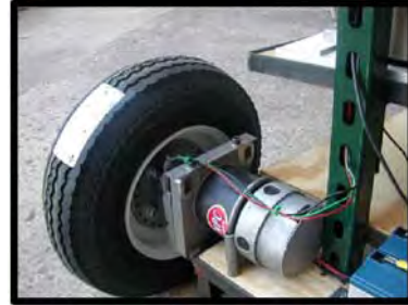
Fig. 9 DC motor and wheel coupling implementation
