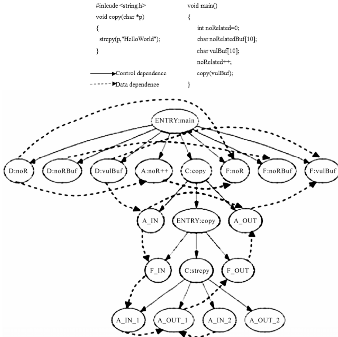
Figure 6. A sample of buffer overflow and its SDG.
