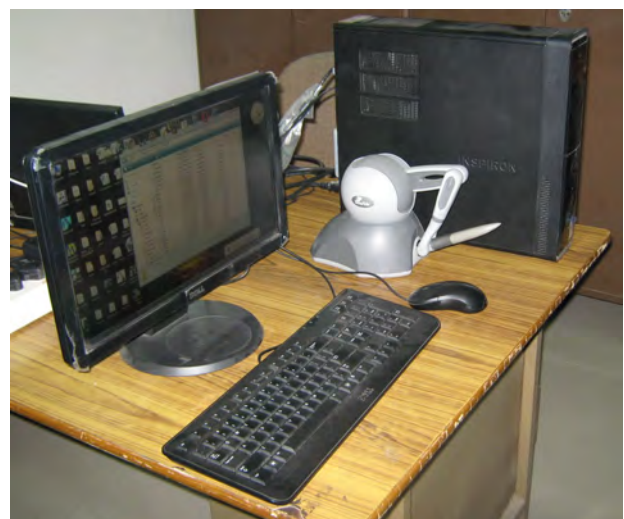
Figure 1. Haptic Rehabilitation Setup with PHANTOM Omni and Computer.
