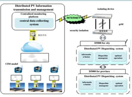
Figure 6. Gridding monitoring system frame of distributed PV.
