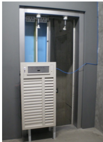
Figure 11. Damper with double blade and vertical duct installed in test bed.
