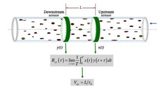
Figure 1. Cross-correlation velocity measurement diagram.
