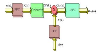
Figure 2. The correlation function calculation in frequency domain.
