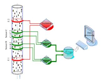
Figure 3. Conductance sensor measuring system.
